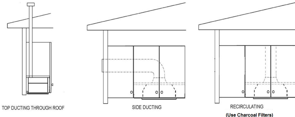
Extra lengths and/or bends may be required, depending on the length required and whether there is any structural material in the run e.g. rafters.
