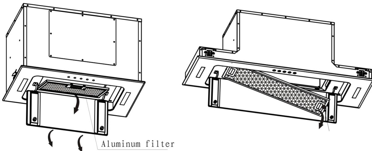
To remove the aluminium filters, first unclip the centre section of the bottom panel and let it swing down. Push in the latch at the handle (see diagrams) and remove. To install, repeat the operation in reverse.
